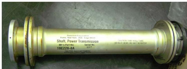
Figure 13 No.2 Engine-to-MGB Coupling Shaft of B-HRN
