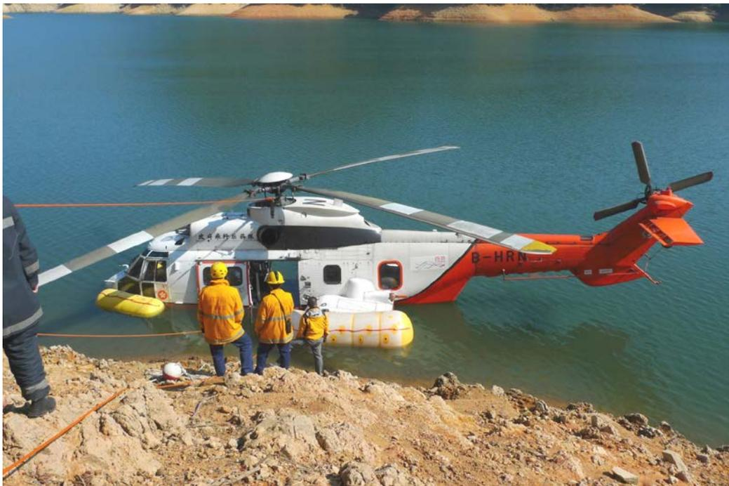
Figure 11 B-HRN on Floats and Secured
