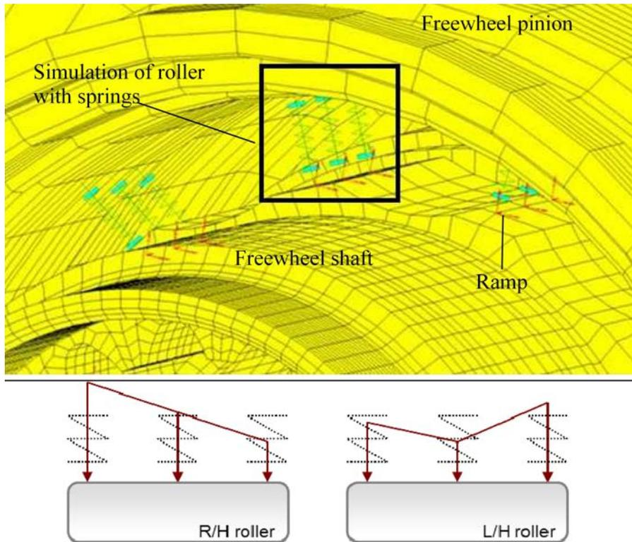
Vertical arrows indicate the load distribution on the rollers.
